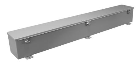
**Construction:** C & I Enclosures Type 12 Hinge Cover Wiring Trough is fabricated in accordance with UL specifications from code gauge steel. An oil resistant gasket is attached to the cover to prevent dust from entering the trough. The cover is attached to the body with butt hinges on one side and external screw clamps on the other. All seams are continuously welded and ground smooth.
